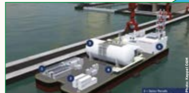
EMA partnered Keppel Offshore & Marine to test-bed Singapore's first floating Energy Storage System. The project will explore a first-of-its-kind battery stacking solution to reduce land take by up to 40%.
