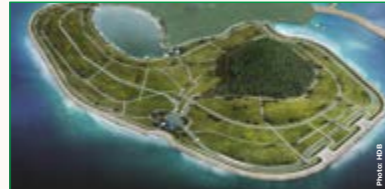
The polder project at Pulau Tekong significantly reduces the need for sand in reclaiming land.
